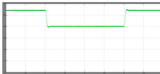
Dc-link current ( I_{dc}, I_{dc\_ref} );
